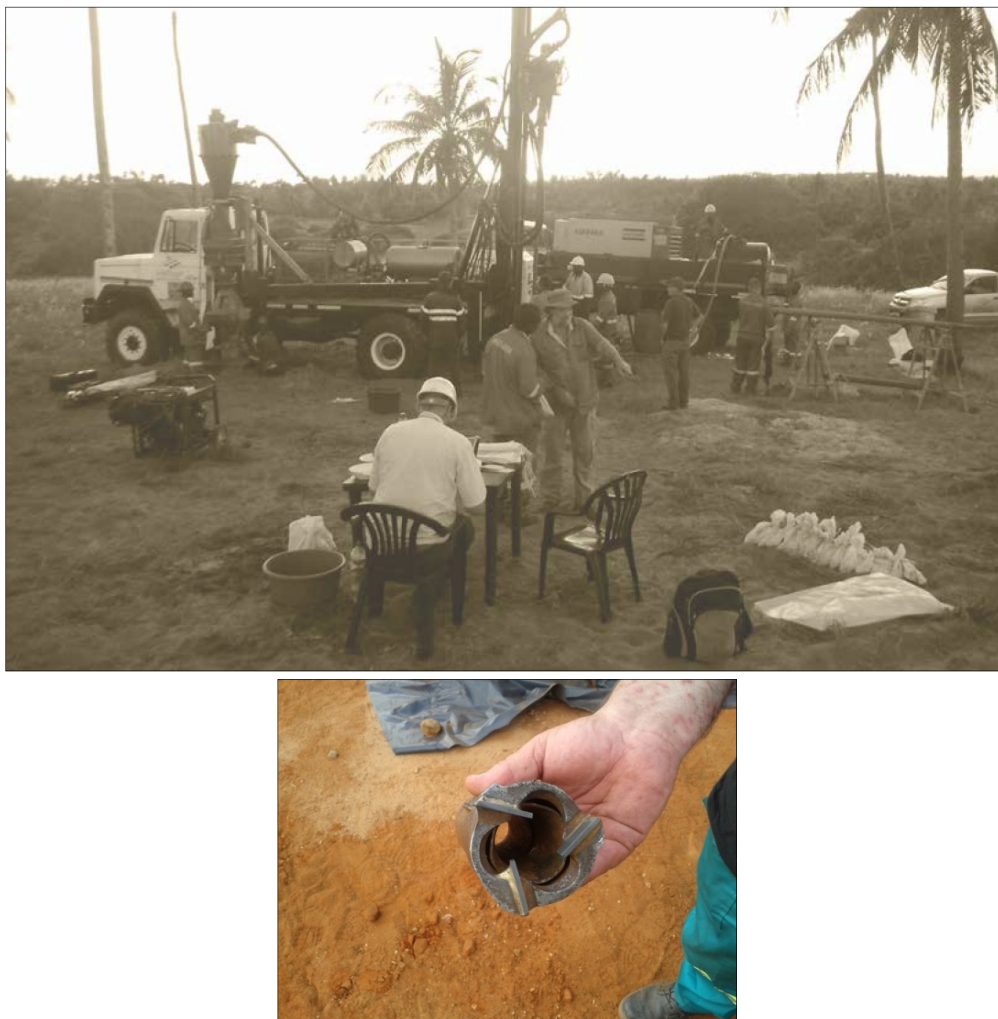
Figure 4.3: Top: drill rig, support truck and cyclone set up on site. Bottom: trumpet style mineral sands air core bit
